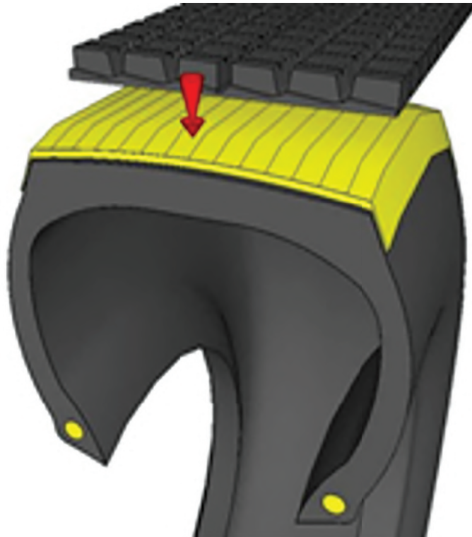
Figure 8 — Retreading operation with a new tread layer
