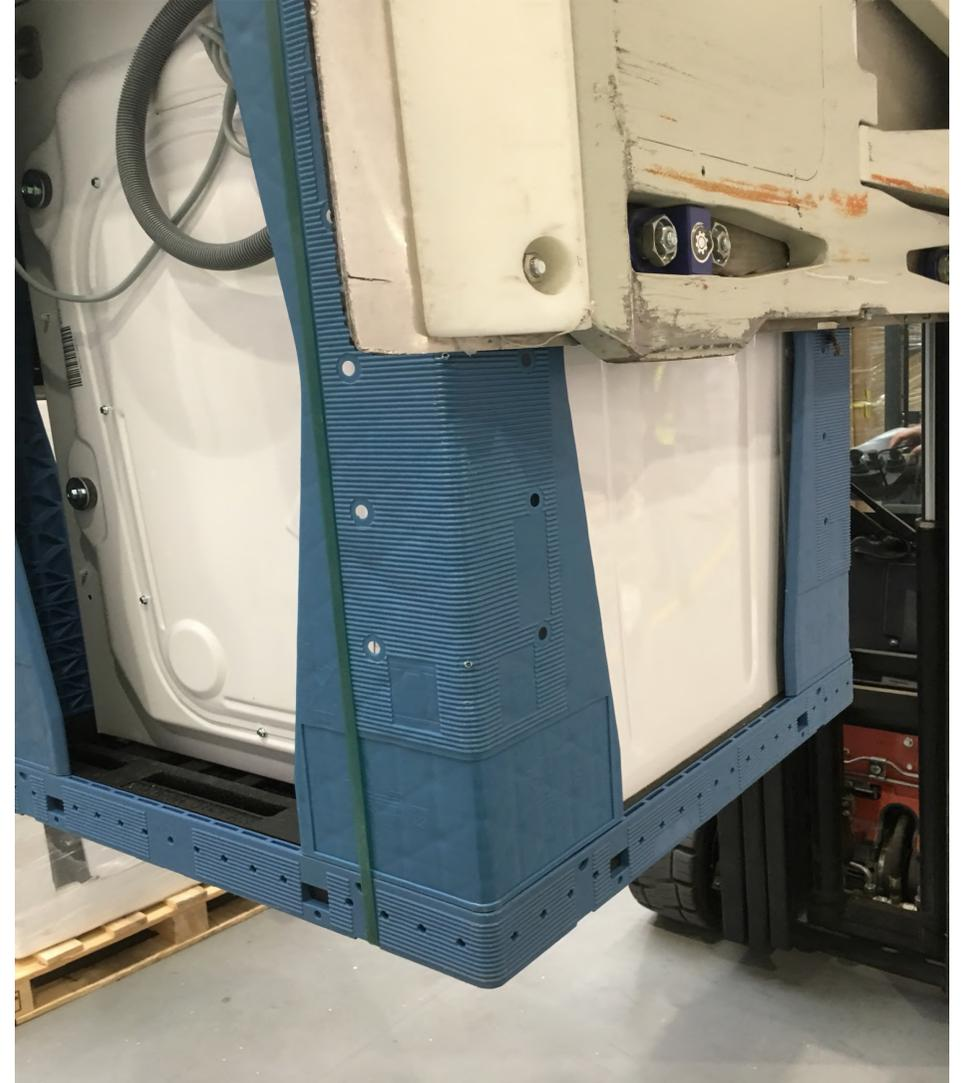
The RPP shell is autonomously able to resist vertical and lateral forces.
